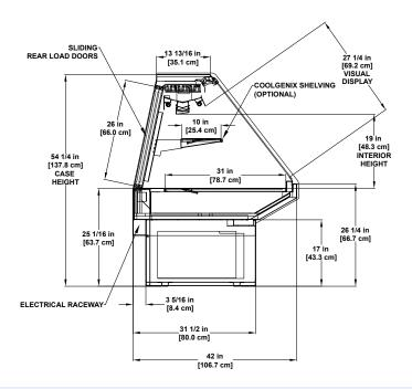
Please consult Hillphoenix Engineering Reference Manual for dimensions, plan views and technical specifications. Specifications subject to change without notice. Designed for optimal performance in store environments where temperature and humidity do not exceed 75° F and 55% R.H. Certified to UL 471 and ANSI/NSF Standard 7.
